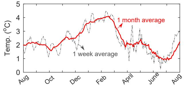
Fig. 6. Temperature difference between the substation and atmospheric temperature.
