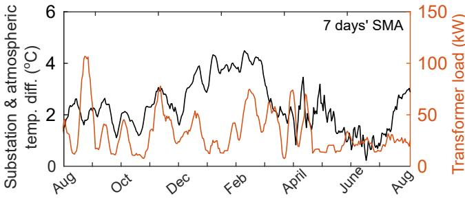
Fig. 5. Difference between the substation and atmospheric temperature vs. different load conditions (average of 7 days' data for a clearer view).
