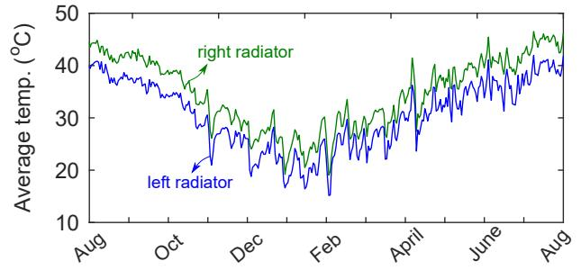
Fig. 7. Temperature profiles of the right and left radiator of the transformer.
