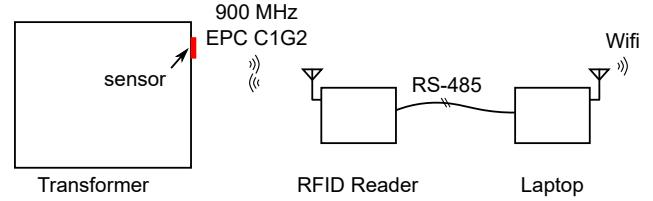
Fig. 2. Illustration of data transmission between different system components.
