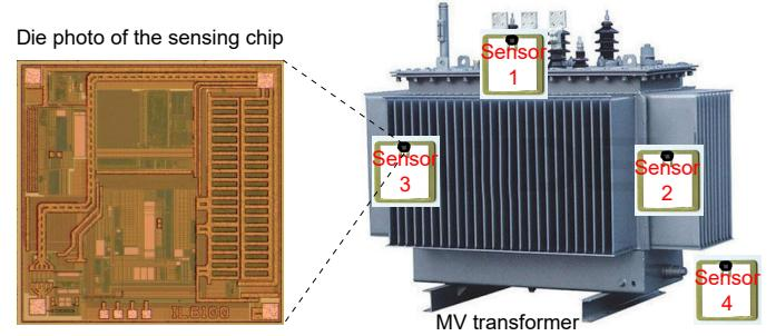
Fig. 1. System block diagram showing the deployment of the sensors (sensor 1: top surface, sensor 2: left radiator, sensor 3: right radiator, sensor 4: hang in the air).
