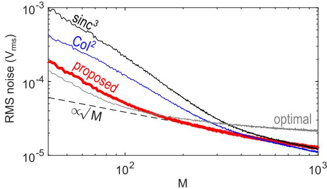
Fig. 15. Measured rms noise of the IDC at different OSRs. The conversion cycles required to reach a thermal-noise-limited state are around 350/300/150 for the  $\text{sinc}^3$ / $\text{CoI}^2$ /proposed decoder, respectively.
