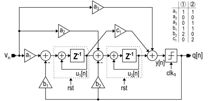
Fig. 11. Generic single-bit second-order  $\Delta\Sigma$  modulator model, together with the modulator coefficients (without signal scaling) for ① the classical CIBF topology, and ② the CIFF structure.
