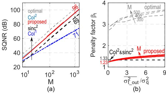
Fig. 7. (a) Simulated SQNR using different filters; (b) thermal noise penalty factor versus the averaged output thermal noise and quantization noise.
