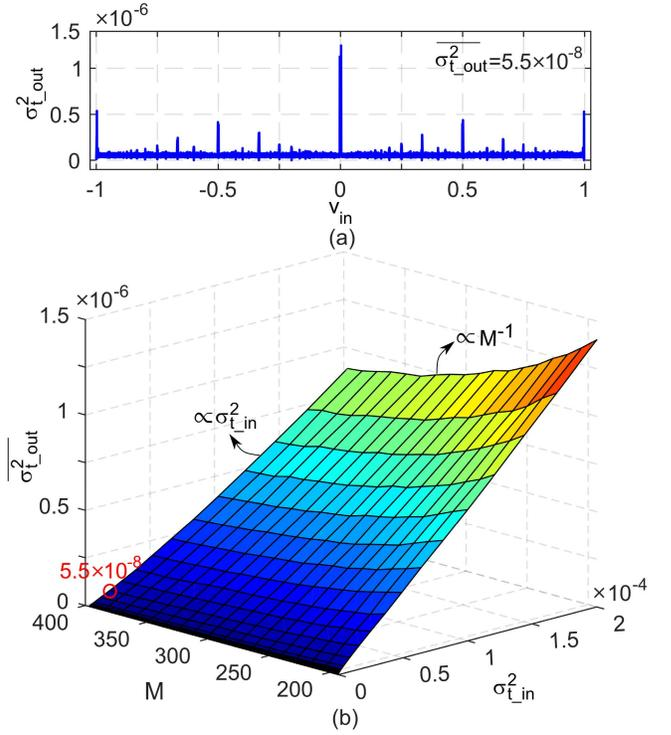
Fig. 8. (a) Output noise for different  $v_{in}$  at an OSR of 397 and  $\sigma_{t,in}^2 = 1.6 \cdot 10^{-5}$ ; (b) averaged output thermal noise for different OSR and  $\sigma_{t,in}^2$  combinations using the proposed decoder.
