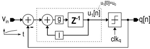
Fig. 9. Nonideal model of a first-order modulator.
