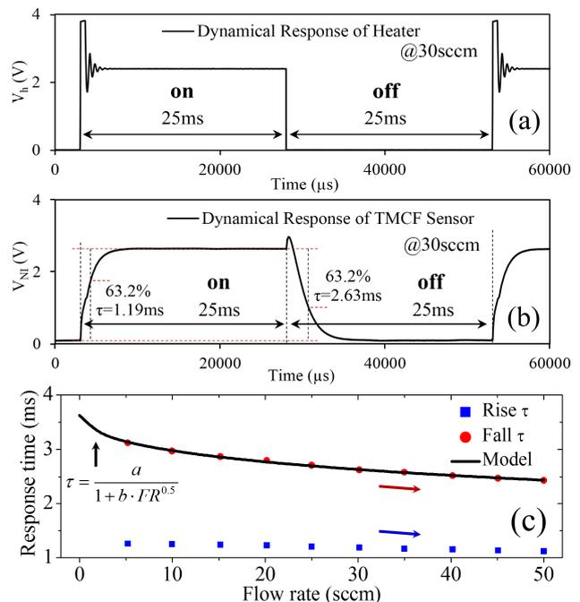
Figure 7. Pulsed operated TMCF sensor (20Hz square wave) in CTD mode with (a) 50% reduced power and (b) time constant  $\tau$  at 30sccm, (c)  $\tau$  vs. flow rates,  $\tau_{\text{max}} < 3.63\text{ms}$ .
