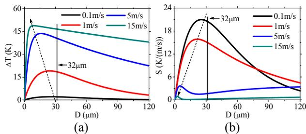
Figure 2. The effect of distance ( $D$ ) between the heater and sensing elements on the TMCF sensor's (a) output and (b) sensitivity, an optimal distance  $D=32\mu\text{m}$  was determined with the 1D model and CMOS MEMS process [7].
