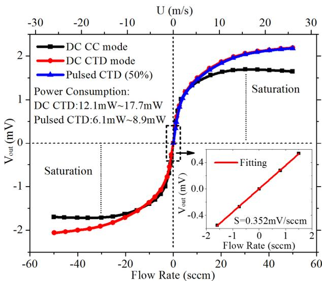
Figure 6. DC and pulsed operated TMCF sensor response to the nitrogen flow  $-50\sim 50$ sccm ( $-26\sim 26$ m/s). The sensitivity is  $0.352\text{mV/sccm}$  and the minimum power consumption  $< 9\text{mW}$ .
